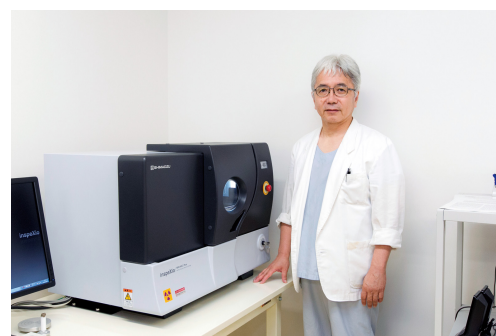
Fig. 10 Microfocus CT system (inspeXio) Used to observe the detailed geometry of bifurcation stents.
